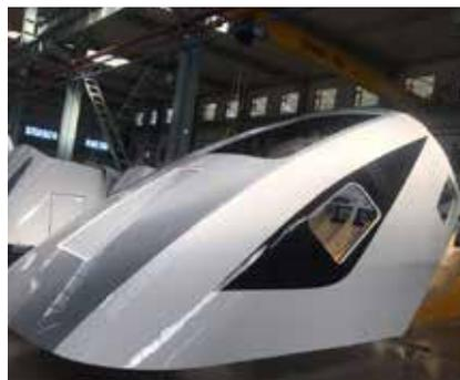
// Nose of the CRH3A bullet train that connects the 700km distant cities of Chengdu and Xi'an in Western China in less than four hours. The success of the CRH3A has put an end to flights between the two cities, thus reducing the carbon footprint on this route.
